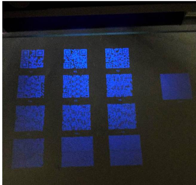
**Figure 3:** Illustrates the printed invisible QR codes were lighted under UV light source (HANDHELD BLACKLIGHT).
