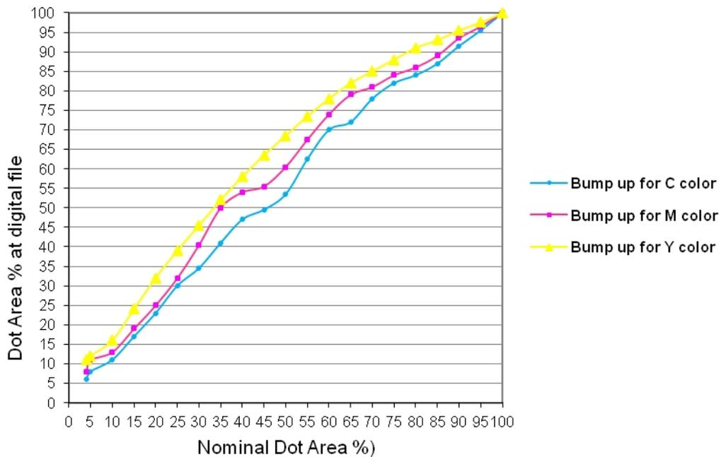
Figure14: the dot areas from 5-100% at digital file after bump up curve for C,M,Y colors
