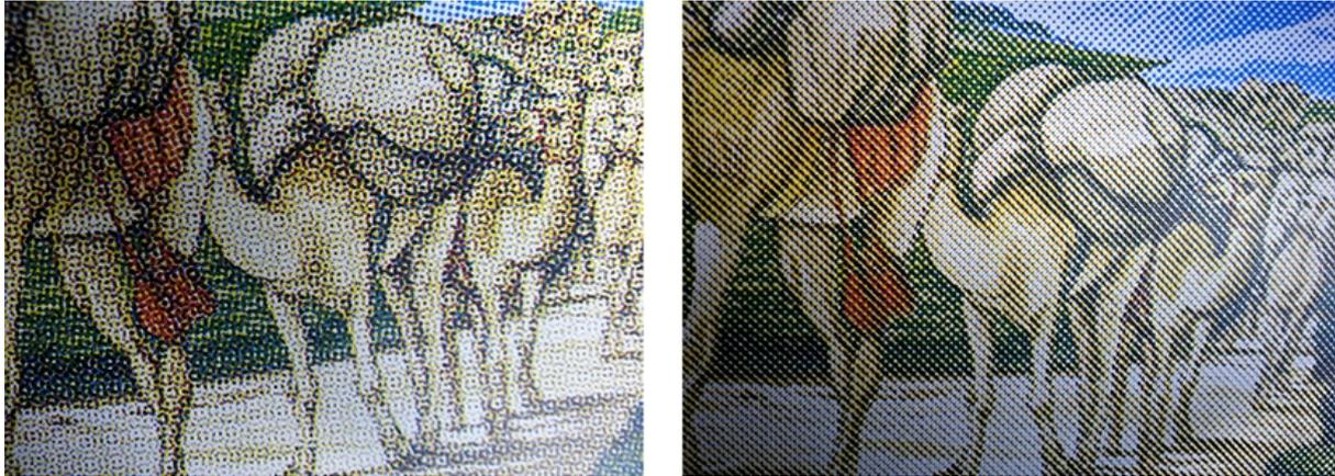
Figure16: enlarged images to compare between images printed using the conventional angles (left) and the same image after processing in pre-press stage (right)
