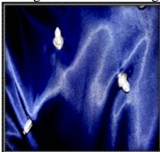
**Fig. (37) LEDs on the satin fabric passing Through grommets.**
