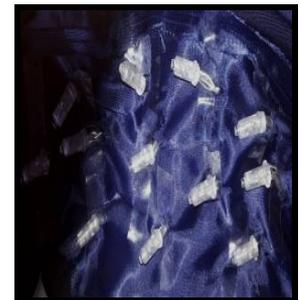
**Fig. (40) LED passing through holes in the satin lining**
