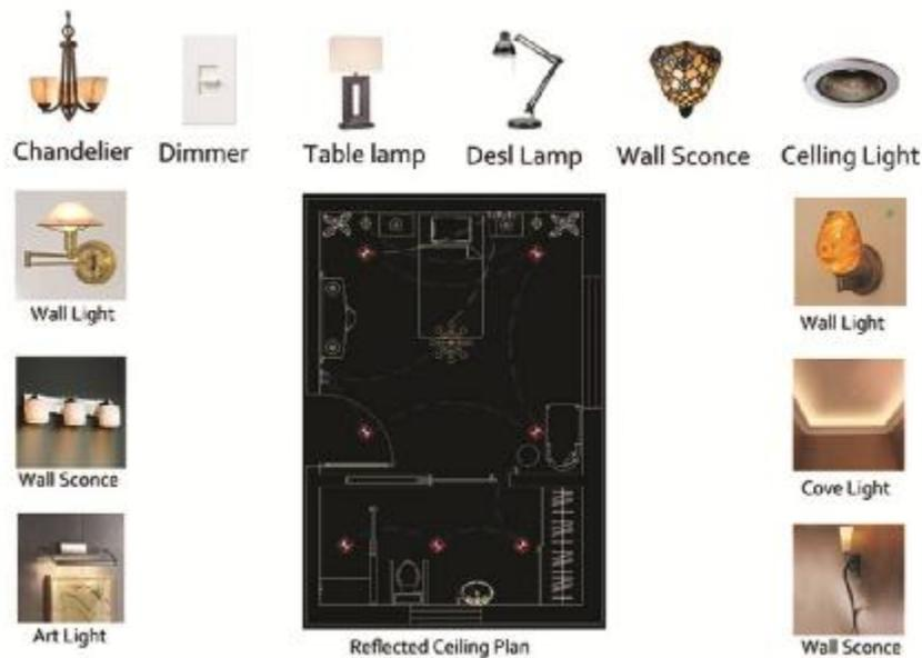
Figure 15: Men's Unit lighting plan & lighting fixtures.
