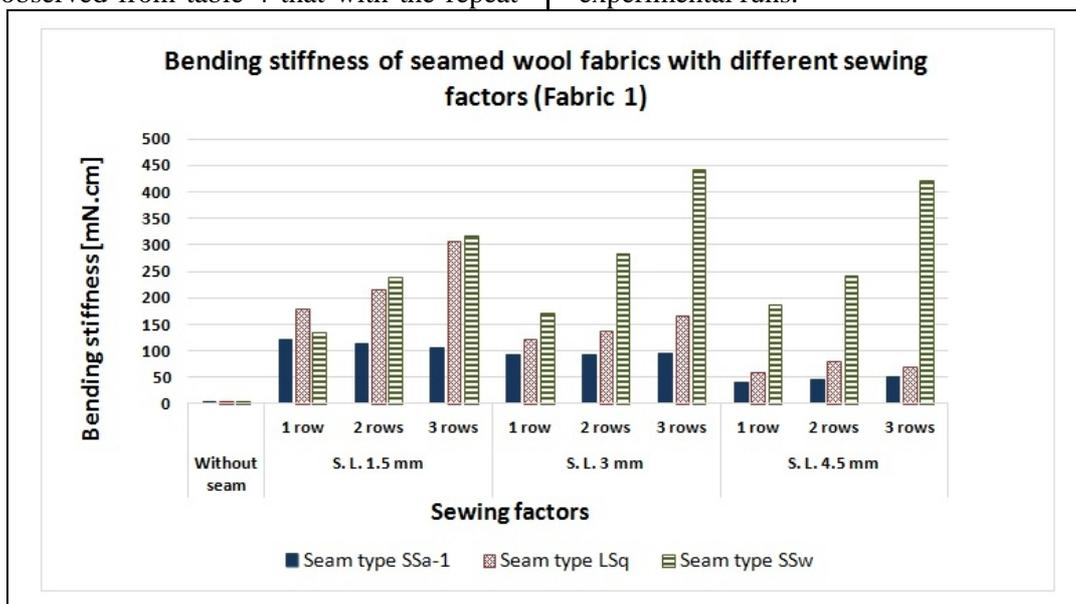
Figure 5: Bending stiffness of fabric 1 with different sewing factors
