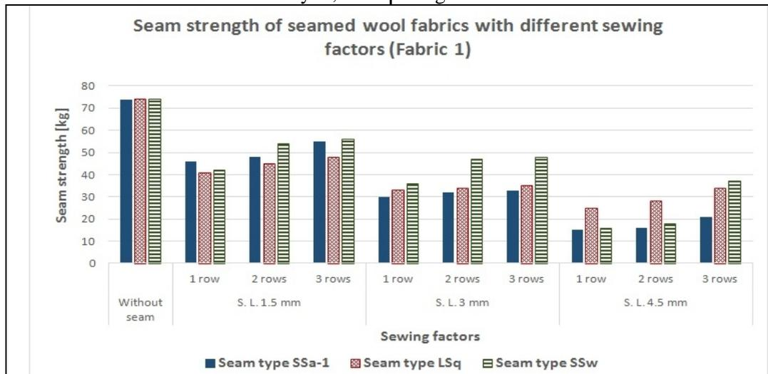
Figure 2: Seam strength of fabric 1 with different sewing factors
