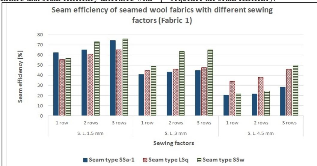
Figure 4: Seam efficiency of fabric 1 with different sewing factors
