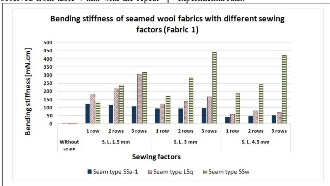
Figure 5: Bending stiffness of fabric 1 with different sewing factors
