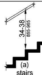
Fig.(12) Height of hand rails
