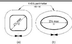
Fig.(11) Handrail cross section
