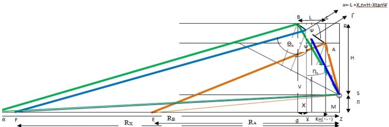
(Fig2-2)Ray diagram shows how and where the acoustical rays hit the reflector surface and study the propagation of direct and indirect sound rays through out the speech closed space.
