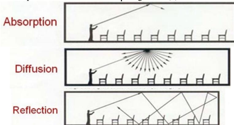
Figure (1-1). Illustration showing how absorption removes the beneficial early reflections from the ceiling; reflection redirects them and diffusion uniformly distributes them for greater coverage and intelligibility.
