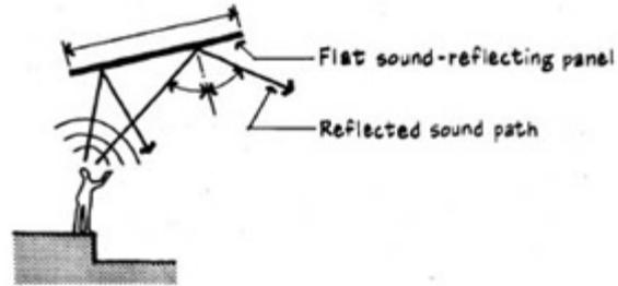
(fig 2-1) inclined reflector, direct sound path and indirect sound path directed from sound source to listener.
