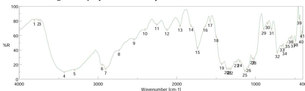
Fig. (11) IR spectrum of natural goat leather (b) treated sample with nano zinc oxide
