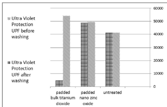
Figure (5) natural goat leather comparison between (untreated, nano zinc oxide, bulk titanium dioxide) samples uv treatment by padding methods
