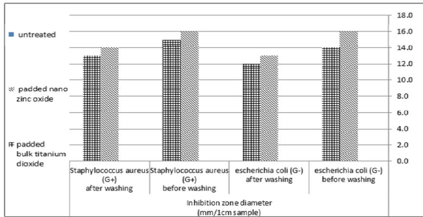
Figure (9) blended 50% cotton, 50% polyester woven fabric comparison between (untreated, nano zinc oxide, bulk titanium dioxide) samples anti-bacterial treatment by padding methods
