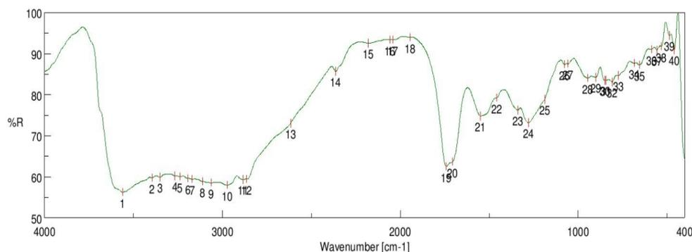
Fig. (8) IR spectrum of natural goat leather (c) treated sample with bulk titanium dioxide
