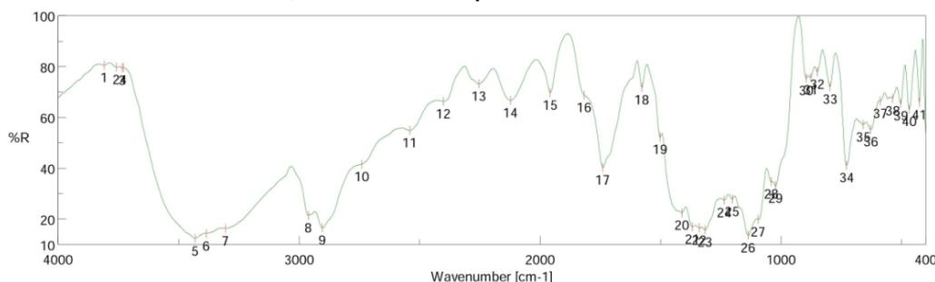
Fig. (10) IR spectrum of natural goat leather (a) Un treated sample
