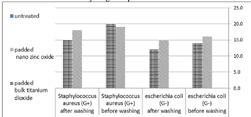
Figure (4) natural goat leather comparison between (untreated, nano zinc oxide, bulk titanium dioxide) samples anti-bacterial treatment by padding methods
