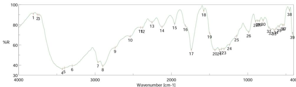
Fig. (12) IR spectrum of natural goat leather (c) treated sample with bulk titanium dioxide
