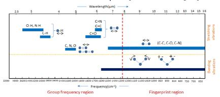
Figure 3. Group frequency and fingerprint regions of the mid-infrared spectrum
