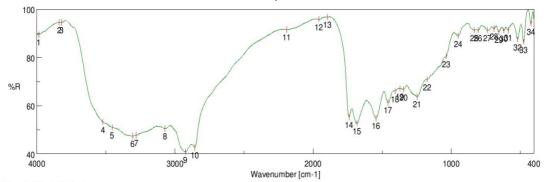
Fig. (7) IR spectrum of natural goat leather (b) treated sample with zinc oxide nanoparticles
