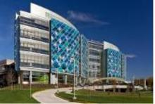
Figure 27:the diagonal pattern and the triangular colors suggest that the glass is modular in that way, they're really rectangular sections of glass that have been twisted with battens on the outside of the building to create the diamond grid.
