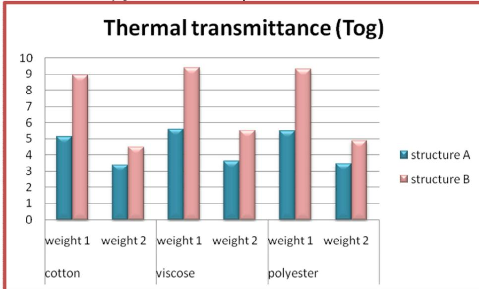
Figure (12) Effect of different weight in wadded nonwoven fiber pad on fabric thermal transmittance
