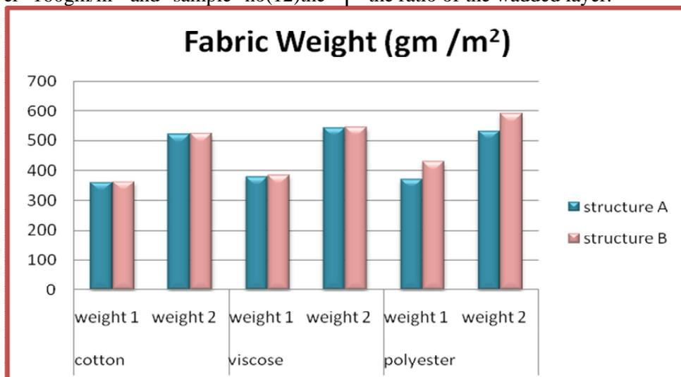
**Figure (10) Effect of different weight of nonwoven fiber pad on multi-layered fabric weight**
