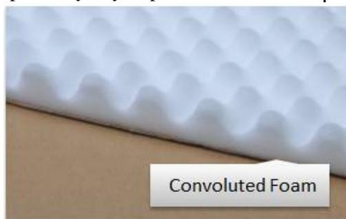
layer of comfort, and may include flat or convoluted PUF as shown in figure (3), shredded pads of compressed polyester, or fiber battings. The insulator and cushioning layers can be stacked in varying sequences between the quilt and the innerspring support.<sup>(3)</sup>
