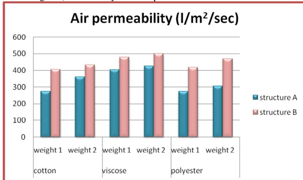
Figure (13) Effect of different weight in wadded nonwoven fiber pad on fabric Air permeability
