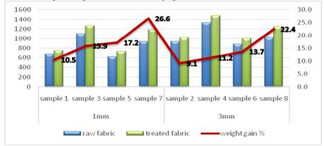
Fig. (5) Relationship between pile length and the weight gain percentage
