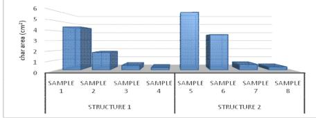
Fig. (7) Relationship between weave structure and flame resistance
