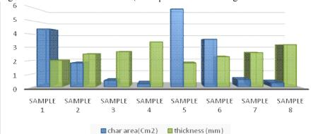
Fig. (11) Relationship between fabric's thickness and flame resistance
