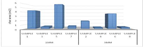
Fig. (8) Relationship between pile length and flame resistance
