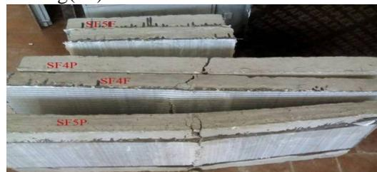
Fig(11):Behavior of Reinforced Slab after Test
