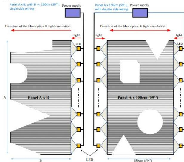
Figure 5 Different ways of cutting the panels, without affecting the lighting effect
