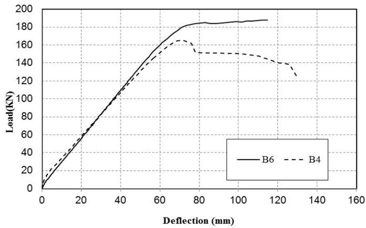
**Fig. 19: Load-Deflection Relationship for B4 and B6**
