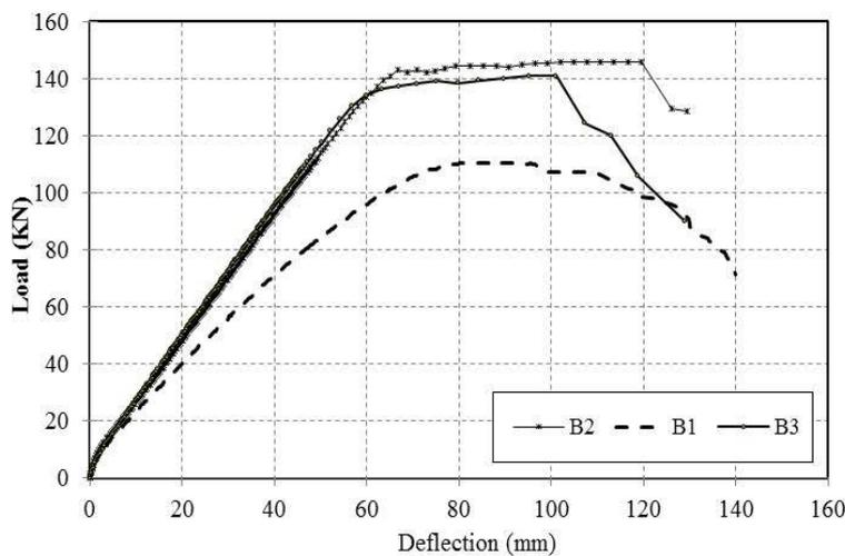
Fig. 15: Load-Deflection Relationship for B1, B2 and B3
