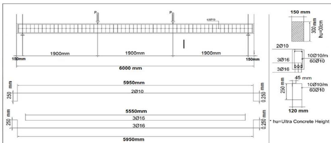
**Fig.1: The concrete dimensions and steel reinforcement details of specimen B1**
