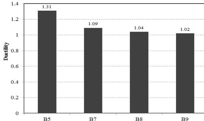
**Fig. 24: Ductility index for B5, B7, B8 and B9**
