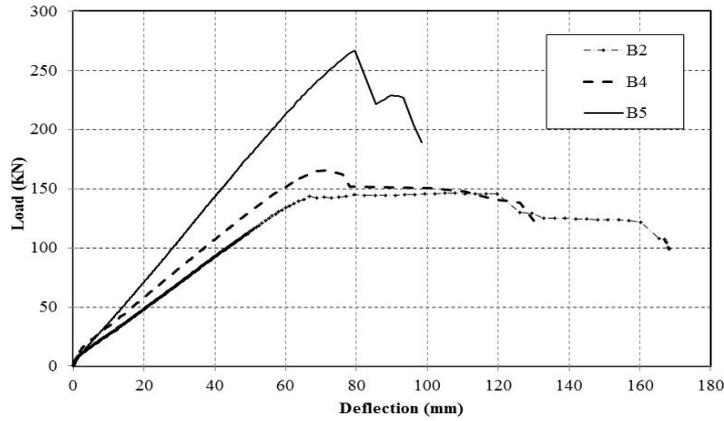
Fig. 7: Load-Deflection Relationship for B2, B4 and B5
