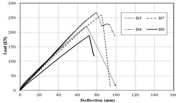
**Fig. 23: Load-Deflection Relationship for B5, B7, B8 and B9**
