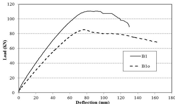
**Fig. 3: Load-Deflection Relationship for B1 and B10**
