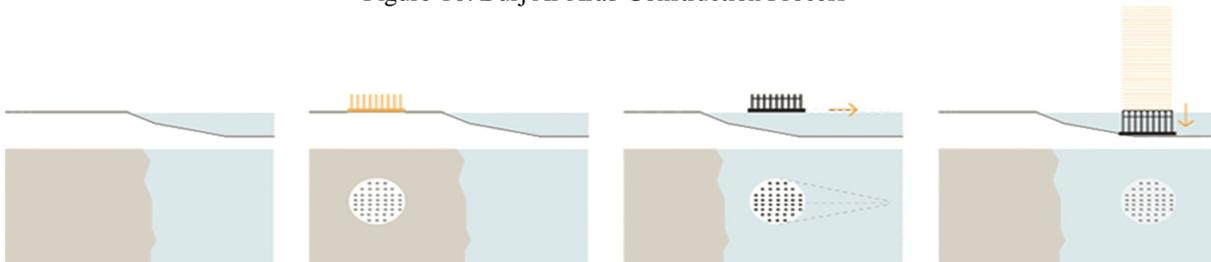
Figure-11: Troll-A Platform Construction Process
