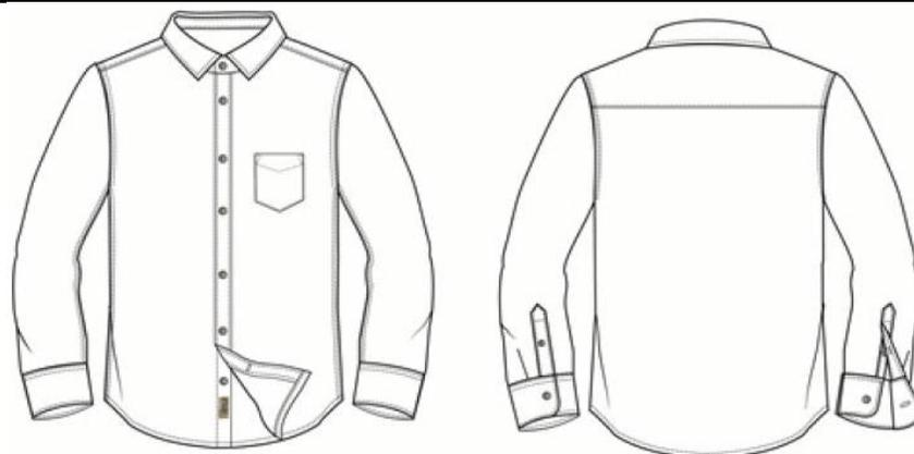
**Figure 1: Technical drawing of the selected model (men's long sleeve shirt)**
