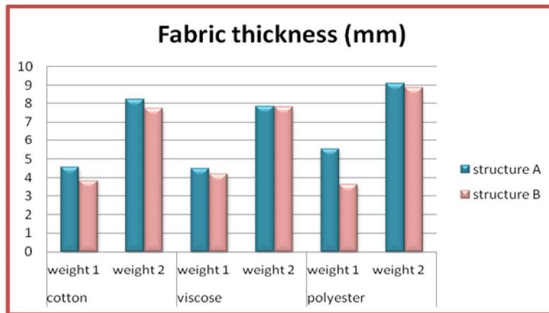
Figure (11) Effect of different weight in the ratio of nonwoven fiber pad on fabric thickness
