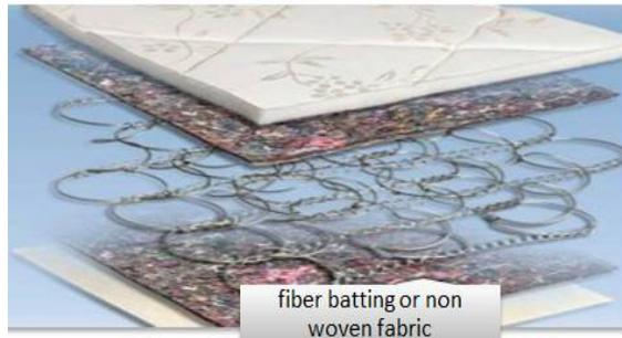
**Figure (2) Mattress cross-section**
