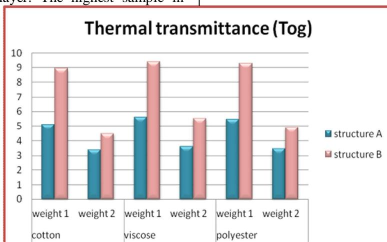
Figure (12) Effect of different weight in wadded nonwoven fiber pad on thermal transmittance
