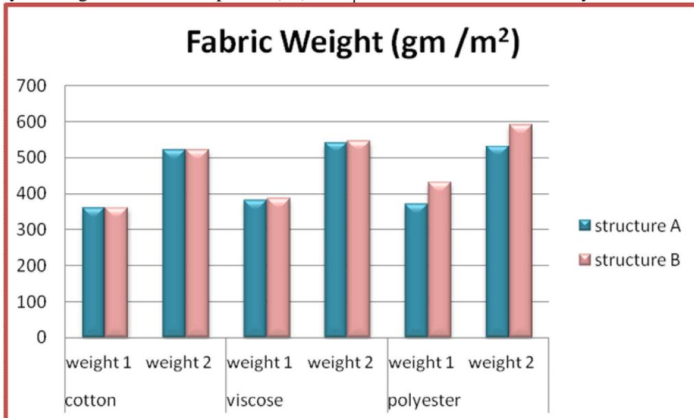
**Figure (10) Effect of different weight of nonwoven fiber pad on multi-layered fabric weight**
