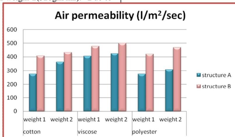
**Figure (13) Effect of different weight in wadded nonwoven fiber pad on fabric Air permeability**
