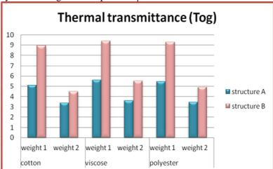
Figure (12) Effect of different weight in wadded nonwoven fiber pad on thermal transmittance
