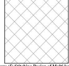
Figure (5) Stitching Design of Multi layered fabric
