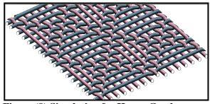
Figure (9) Simulation for Honey Comb weaves 2.3. Laboratory Tests Applied to Samples under Study
