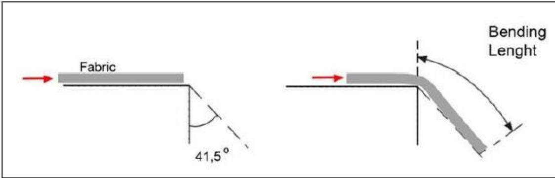
Figure 4: Bending length determination [1]
