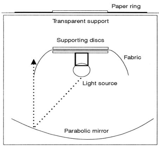
Figure 2: Principle of Cusick drape meter tester [4],[6]
