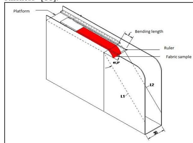
Figure 3: bending stiffness according to Cantilever method [16]
