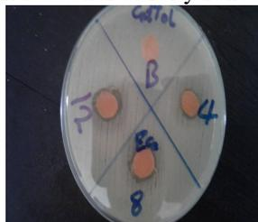
Antibacterial activity zone of inhibition E. coli of fabric bamboo treated with chitosan
