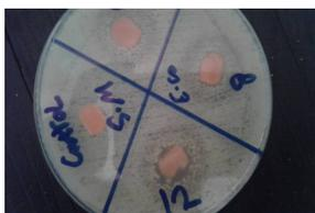
Antibacterial activity zone of inhibition *E. coli* of fabrics bamboo70 % & cotton 30% treated with chitosan
