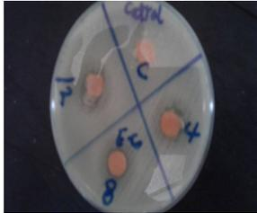
Antibacterial activity zone of inhibition *E. coli* of fabric cotton treated with chitosan
