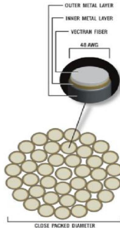
Fig. 1 Across-section of nickel Conductive yarns Lebrator 40 KururayVectran®
