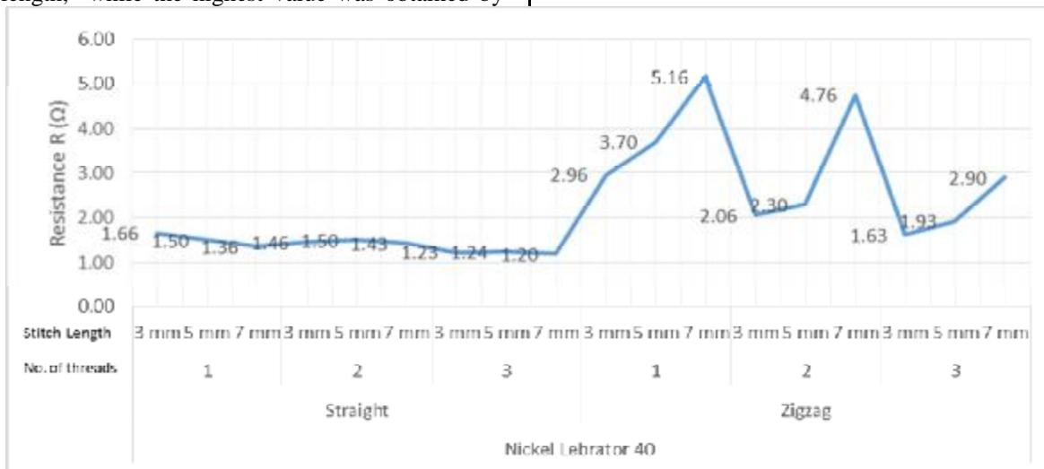
Fig. 5 Effect of yarn type, stitch type, No. thread and length (mm) of stitch on  $R(\Omega)$
