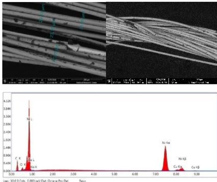
**Fig.4 SEM Micrographs and EDX spectrum of Nickel conductive yarn.**
