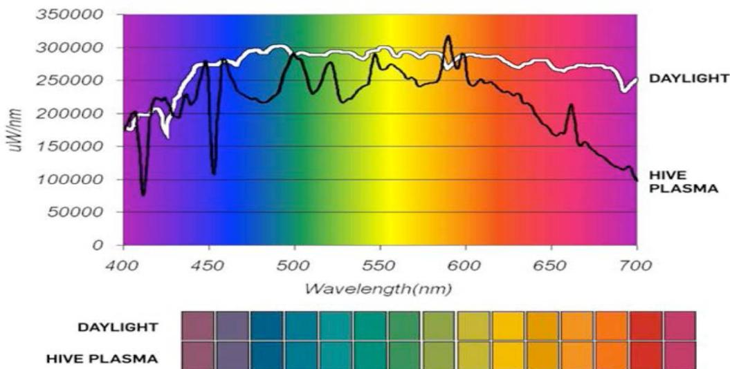
Figure 10 the spectral color distribution for the Plasma light and the Daylight
