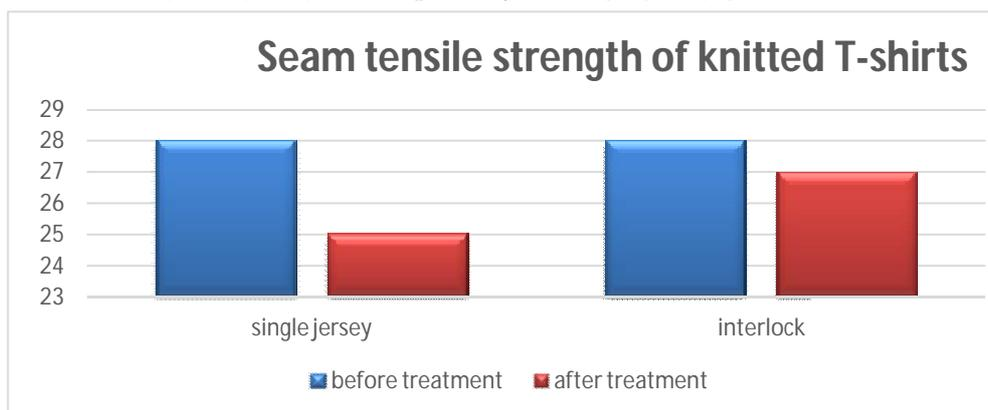
Figure 3. Effects of cellulase enzyme on seam tensile strength of side seam of different knitted T-shirts.
