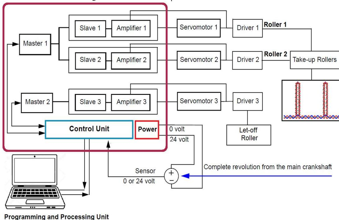
**Fig. 7:** Control system block-diagram for the movement devices on the weaving machine (inter-fabric) is 20 mm, and the length of the pleated length (Wrinkle) is 20 mm. The woven pleated length was 40 mm; it would be 20 mm
