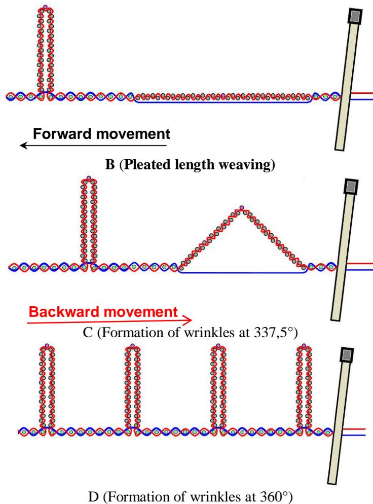
**Fig. 5:** The weaving technique phases of pleated fabric
