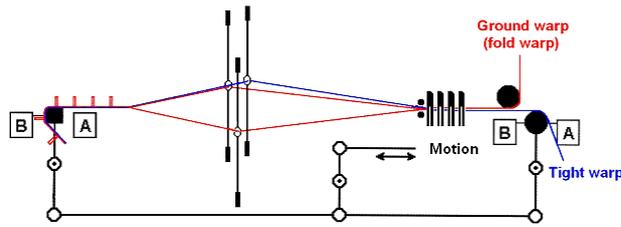
Fig. 2: Device for pleated fabrics weaving /5/
