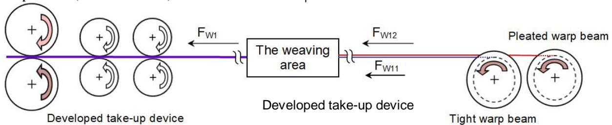
**Fig. 10:** The developed take-up device (forward motion)
