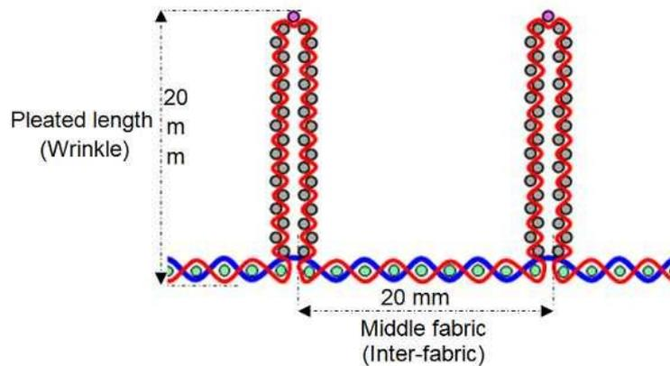
**Fig. 8:** Structure-geometry of the pleated fabric sample
