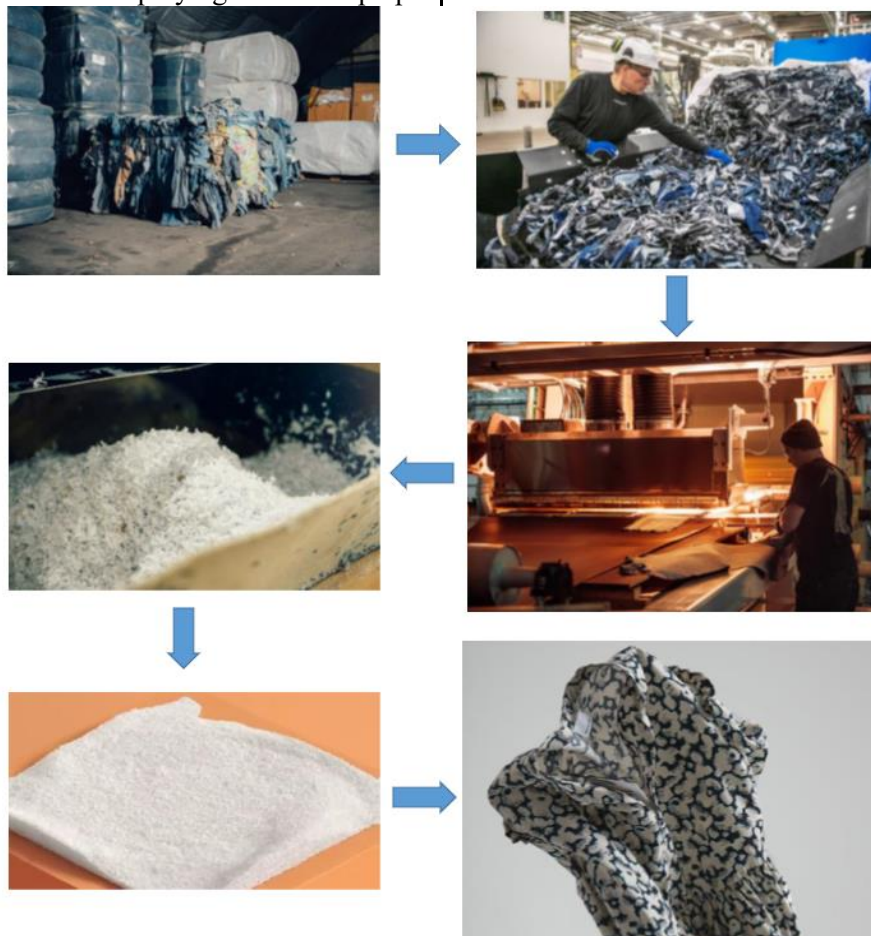
Fig. (4): Steps of converting textile waste into recycled fibers (10)
