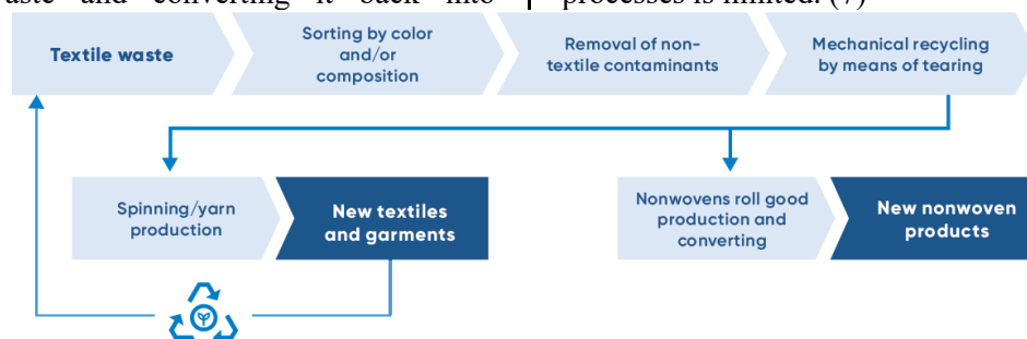
Fig. (2): Recycling process based on mechanical recycling (8)
