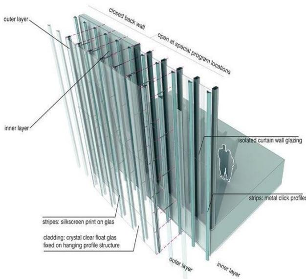
**Figure (6) The lighting design was developed in parallel with the architecture and capitalizes on the double layered facade structure.**
