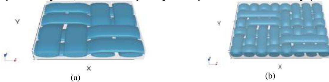
Figure (1) 3-D Simulation of (A) Matt Rib 2/2 and (B) Bique Weave Structure Modeled in TexGen
