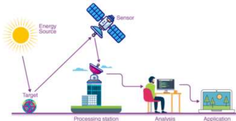
Figure 6: Remote sensing mechanism.
