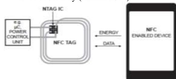
Figure (7) NFC tag interacting with device capable with NFC
