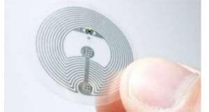
Figure. (11) The NFC Labels is covered with a plastic layer.
