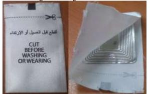
Figure. (10) NFC Labels attached to clothes, written on it "cut before washing or wearing".
