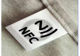
Figure. (12) NFC Label Design and attach it to the clothes.
