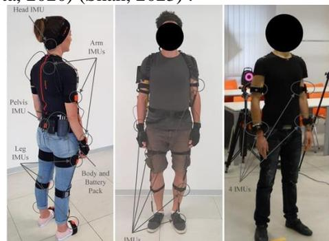
Figure (14) Wearable sensors worn by volunteers. Wearable sensor technology measures movement and acceleration using single or multi-axial accelerometers; it also collects data on temperature, pressure, image analysis, GPS, gyroscopes, and magnetometers. Numerous sectors, including
