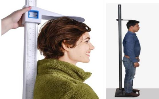
Figure (4) Stadiometers for measuring body heights
