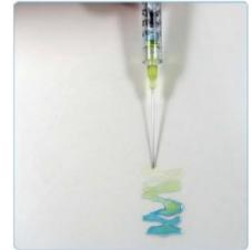
Figure 13: Demonstration of indicator color change after exposure to oxygen
