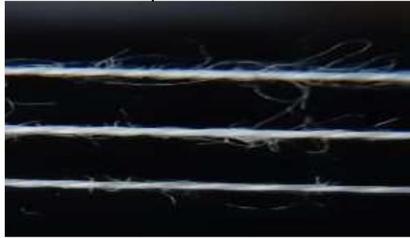
Fig.1 Microscopic photograph of the difference in hairiness between, untreated(a), S(b), and SM(c) cotton yarns
