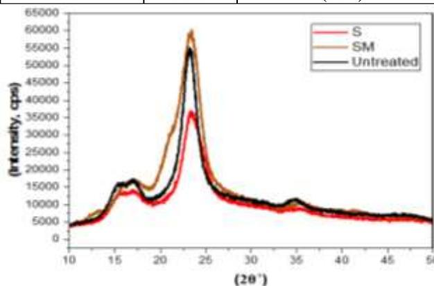
Fig. 5 XRD of untreated, S, and SM of cotton yarns
