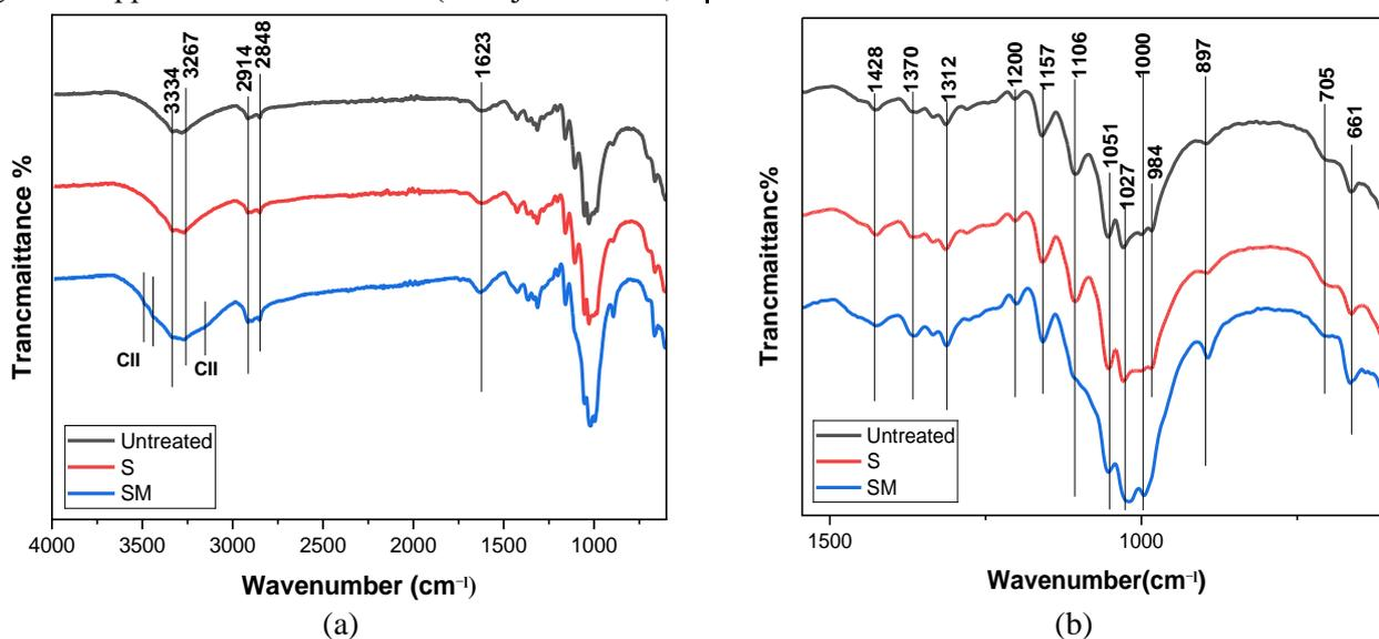
Fig.3 FTIR of the untreated, S and SM of cotton yarns
