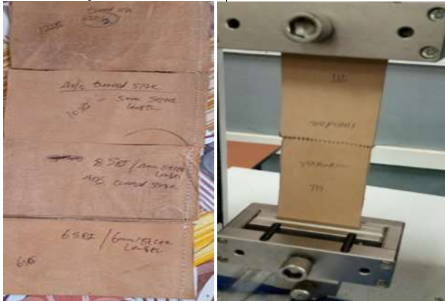
Figure 2 Stitched Samples and Seam Strength Test of Cow Upper Leather
