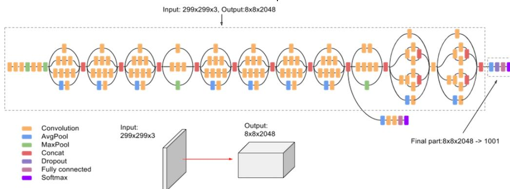
Figure 2. A high-level architecture of the Inception v3 model, to make it run efficiently on the cloud [ <https://cloud.google.com/tpu/docs/inception-v3-advanced> ].
