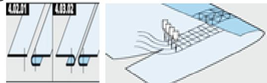
Fig. (6) Superimposed Seam (SS) sewing
