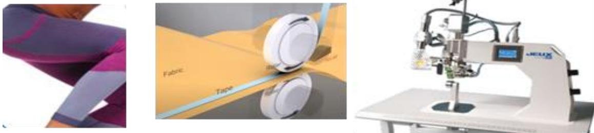
Fig. (2) Ultrasound sewing using Tape Bonding / Seam Sealing
