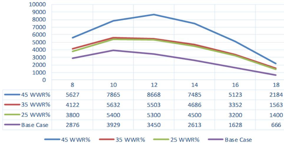
Figure 18: Comparison of the Max Illuminance(lux) graph for the base case and Improved case
