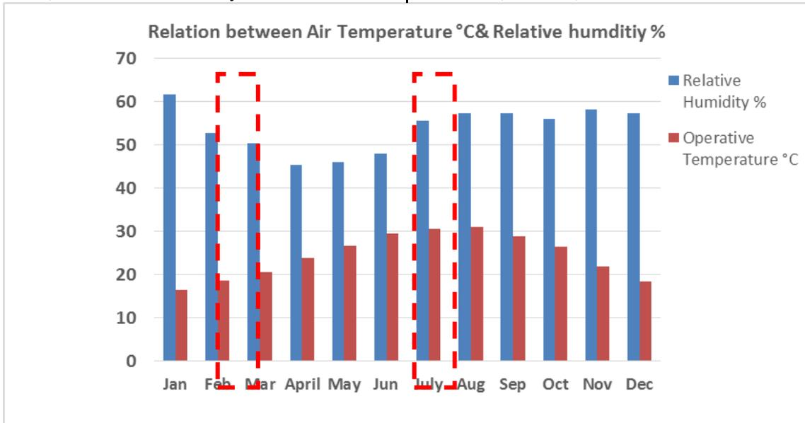
Figure 8: Relation between the Operative air temperature OC and relative humidity % of the Base case
