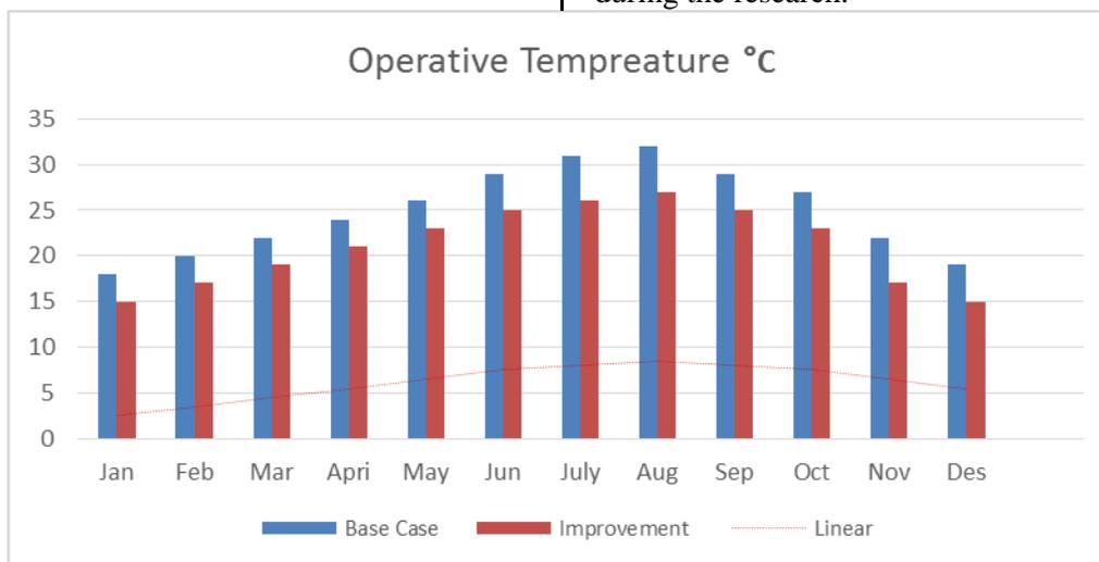
Figure 17: Comparison of the operative air temperature OC for the base case and Improved case
