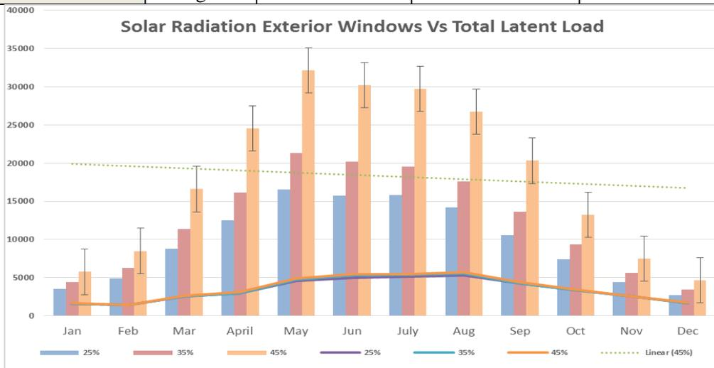
Figure 19: Relation of solar radiation exterior window and total latent load of the Improved case
