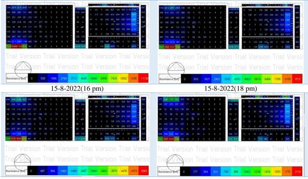
Table 7. Daylighting illuminance(lux) Grid Outputs of the Design-builder Simulation of the different hours of the Base cases on August 15th.
