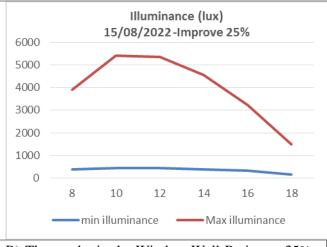
B) The results in the Window Wall Ratio are 35% between the 15th of August and the 15th of March for daylight hours (8 am, 10 am, 12 pm, 14pm, 16 pm, and 18 pm).
