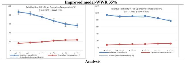
According to the graph, the adaptation of the retrofitted strategies, the maximum operative air temperature is 22 OC at 6:0 pm with 58 % RH.
