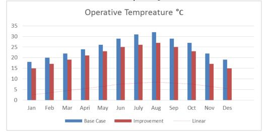
Figure 17: Comparison of the operative air temperature OC for the base case and Improved case
