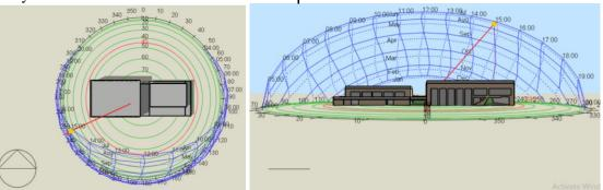
Figure 6: Solar path of the sports hall building, Cairo, Egypt, Source: Design builder by Authors Table 3: Design Builder Simulation input parameters
