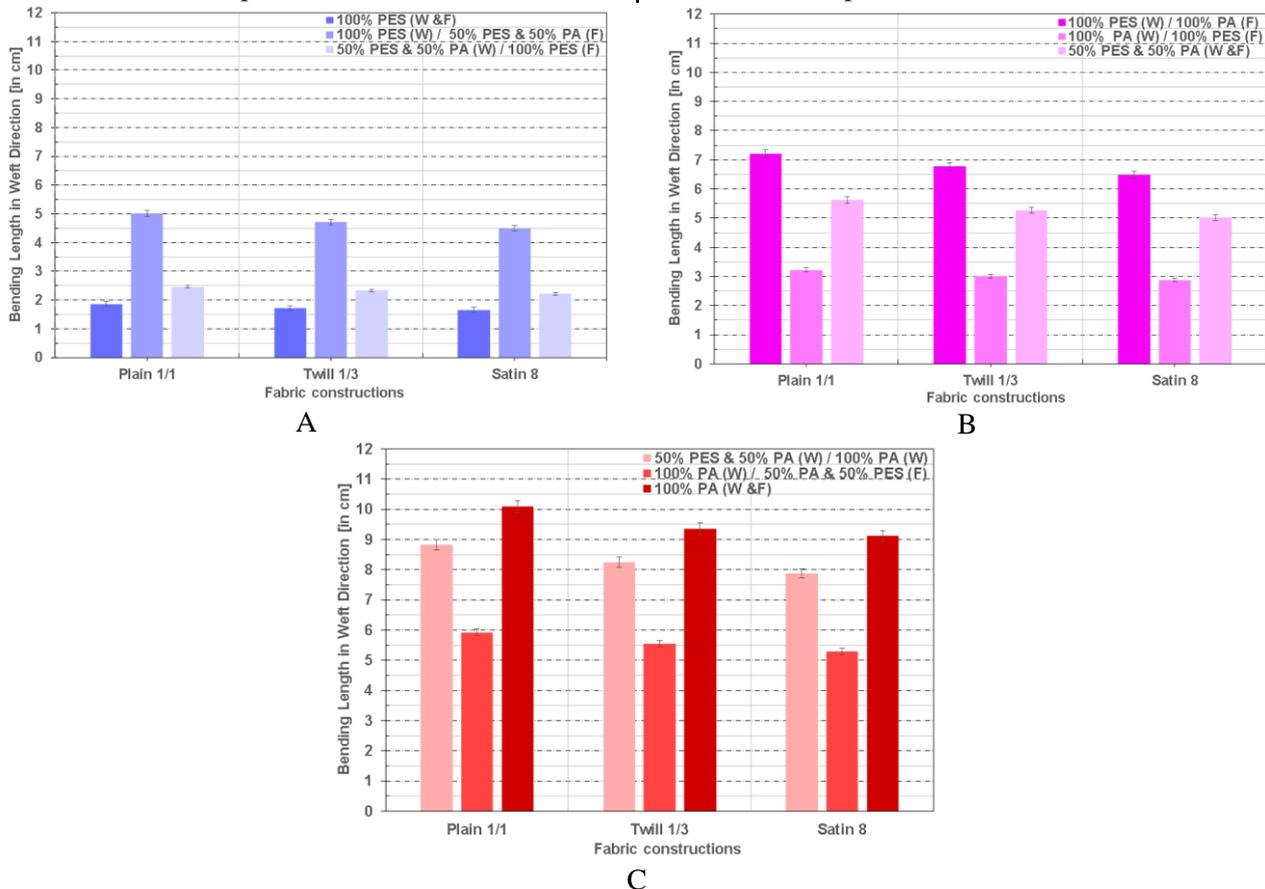
Fig. 4: The relation between fabric construction elements and bending length in the weft direction
