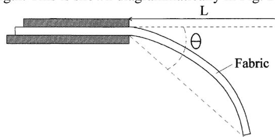
Fig. 2: Bending length (Peirce's cantilever) test / 5, 6/
