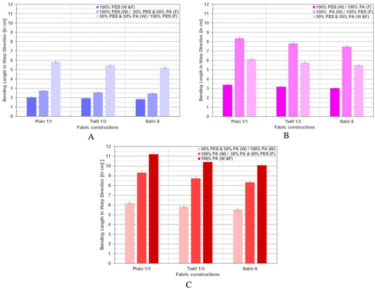
Fig. 3: The relation between fabric construction elements and bending length in the warp direction
