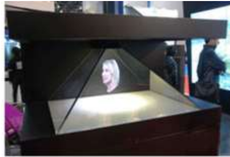
Shape no. 7 It shows how the hologram is displayed inside the glass box, where the display is inside a tetrahedral glass pyramid.
