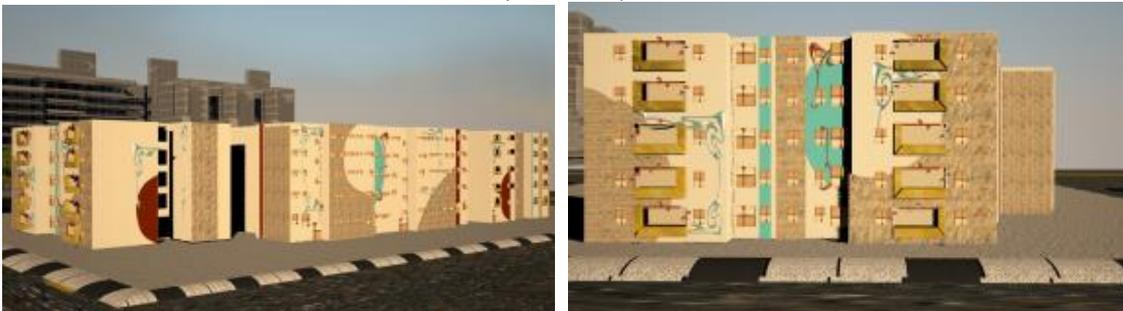
The design with variety of material textures of the external cladding and the use of stone materials to overcome the weather conditions and environmental factors also using of color in simple decorative forms (elmougy 2018)
