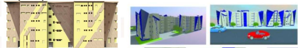
Decorative designs with addition : on the right light protrusions to confirm the decorative formation of the facade using lines at diagonal angles to treat the boredom and monotony of the design ... The external cladding is made of cement raw materials to face weather factors.
