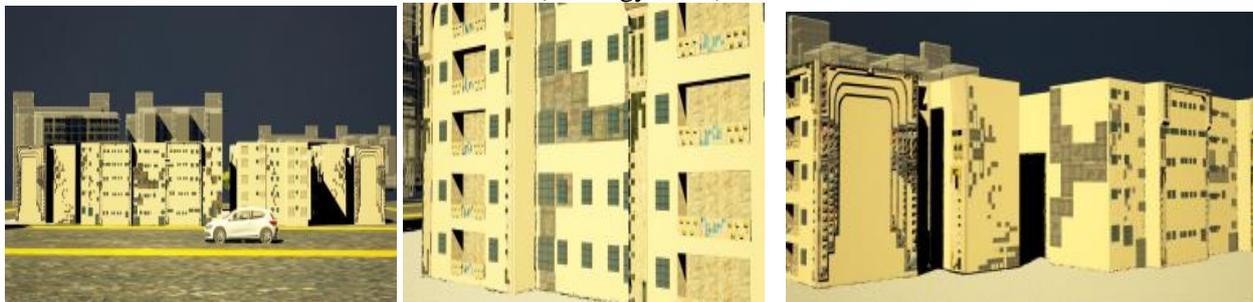
Designs using decorative tiles with a change in the shape of windows, architectural openings . Tiles made of natural materials in their natural colors. The design comes from the arrangement of these tiles, as well as variety and the possibility of making grouped formations (elmougy 2018)
