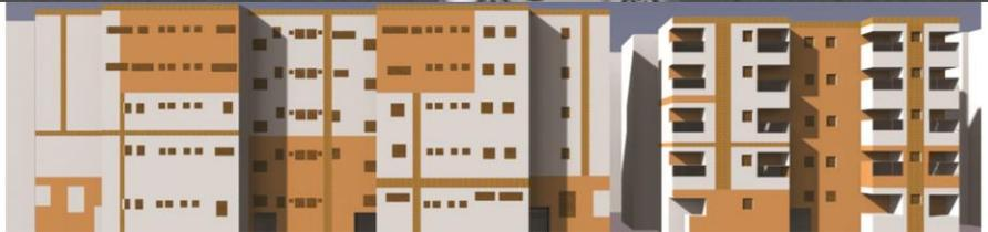
The designs above use vertical and horizontal straight lines to deal with the problem of pipes in the facade and add shapes to them prominently with changing of colors matching with surrounded environment (debsy 2018) .
