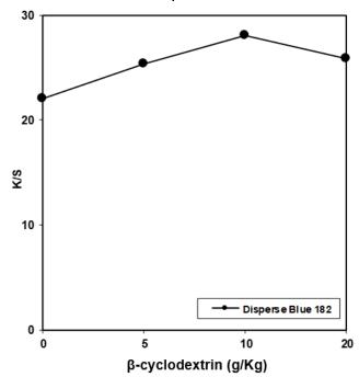
Fig.1. Effect of incorporation of  $\beta$ -cyclodextrin on K/S of the obtained prints into disperse printing. Disperse Printing formulation: Disperse dye (20g/Kg); Sodium alginate (10%) (500g/Kg); citric acid (10 g/Kg); Arkofix® NDF (10g/Kg);  $\beta$ -CD (0-20g/Kg); PEG-600 (20g/Kg). Drying followed by steam fixation at 120 °C/20min.
