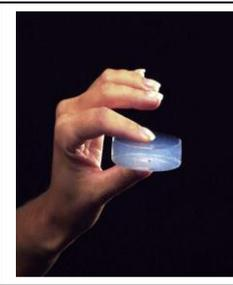
**Fig. 5:** silica aerogel (Monolithic) <sup>(4)</sup>.
