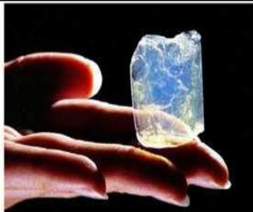
**Fig. 6:** Aerogel, the world's lightest solid <sup>(5)</sup>
