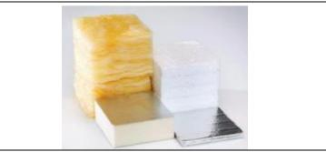
Fig. 15: Different insulating material thicknesses compared to attain the same U-value.<sup>(14)</sup>
