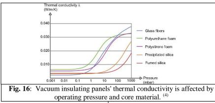
• Vacuum insulating panels (VIPs) now hold the <u>record</u> for thermal insulation with thermal resistance values up to 20 times greater than typical insulating materials such as polystyrene foam or mineral wool. (Fig. 16)
