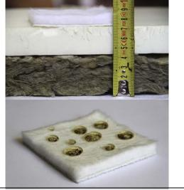
Fig. 8: The relationship between thermal conductivity<br/>and operating temperature in insulating materials <sup>(2)</sup>.Fig. 9: Rock wool, polyurethane, and fiber-<br/>reinforced polymer thickness comparison <sup>(2)</sup>Table (1) Aerogel vs. conventional insulating materials <sup>(2)</sup>
