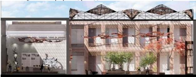
Figure 10. Section demonstrating the atrium and the gallery showing the use of hollow brick tiles and the use of glass covering the inner courtyard area as a principle of sustainability. The solar glass is characterized by three distinct mechanisms: reflection, absorption, and permeability. (Option 1)
