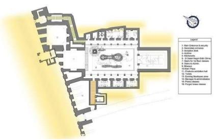
Figure 7. Plan of the First floor demonstrating functional relationship (Source: From the work of the
