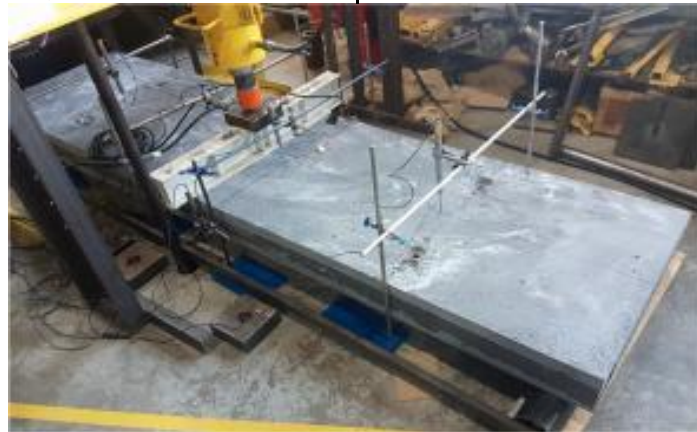
Fig. 8 Instrumented panel in place for structural testing [16]
