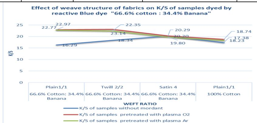
Fig. (11): Effect of weave structure of fabrics on K/S of dyed samples with Reactive blue in presence and absence of plasma treatment.
