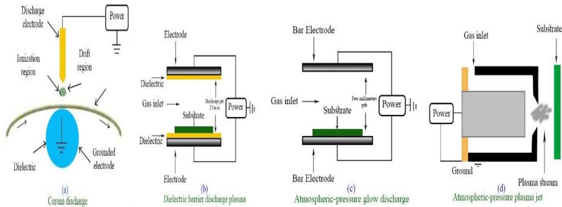
Fig. 3 Schematic illustration of various atmospheric-pressure plasma treatments on textiles: CD (a), DBD (b), APGD (c), and APPJ (d)
