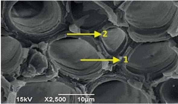
Figure (2) . SEM image of banana pseudo-stem fibre. [6]
