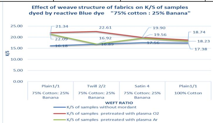
Fig. (10): Effect of weave structure of fabrics on K/S of dyed samples with Reactive blue in presence and absence of plasma treatment.
