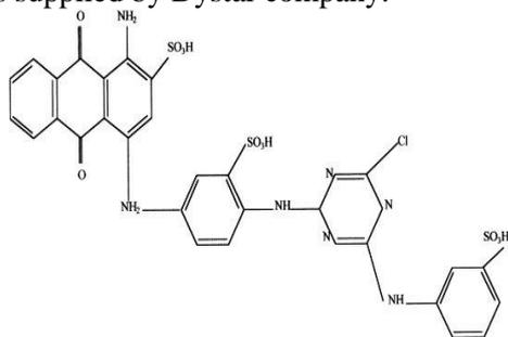
Figure 4. Chemical structure of levafix red.
