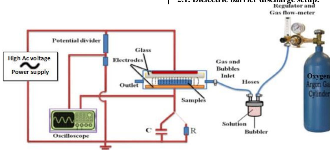
Figure 6 shows a schematic diagram of the DBD reactor used to treat samples.
