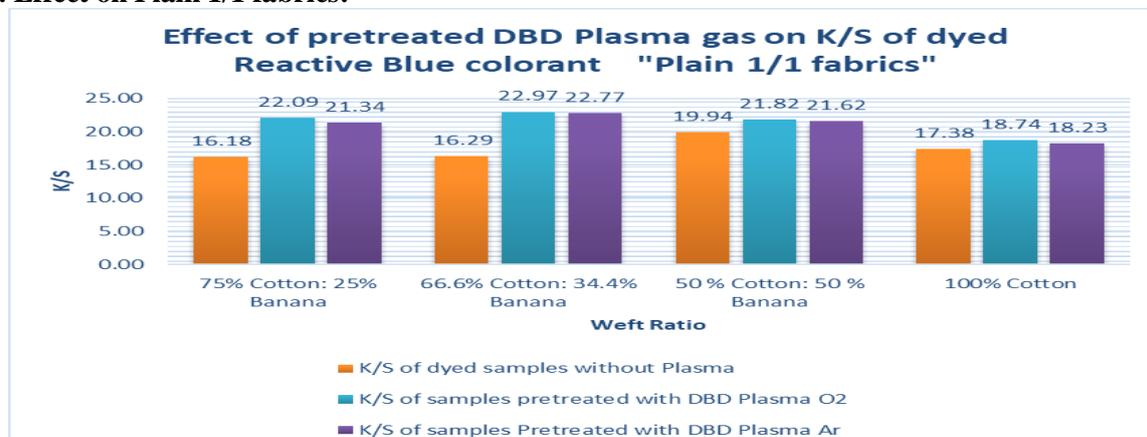
Fig. (7): Effect of using Pre-treatment plasma on dyeing plain fabrics with reactive Blue dye in presence of different gases
