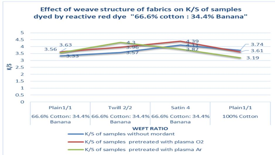
Fig. (17): Effect of weave structure of fabrics on K/S of dyed samples with Reactive red in presence and absence of plasma treatment.
