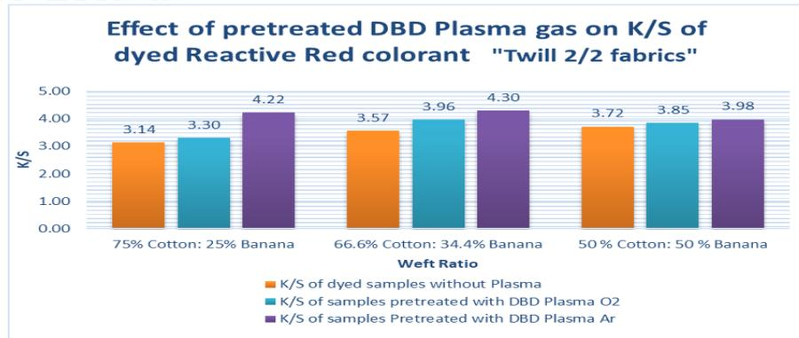
Fig. (14): Effect of using Pre-treatment plasma on dyeing twill 2/2 fabrics with reactive Red dye in presence of different gases.
