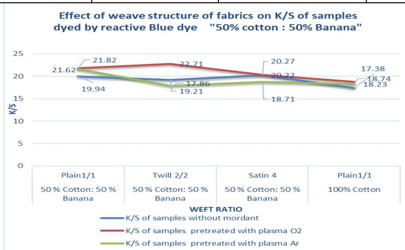
Fig. (12): Effect of weave structure of fabrics on K/S of dyed samples with Reactive blue in presence and absence of plasma treatment.
