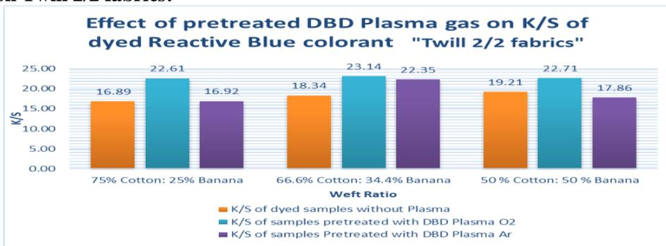
Fig. (8): Effect of using Pre-treatment plasma on dyeing Twill 2/2 fabrics with reactive Blue dye in presence of different plasma gases.
