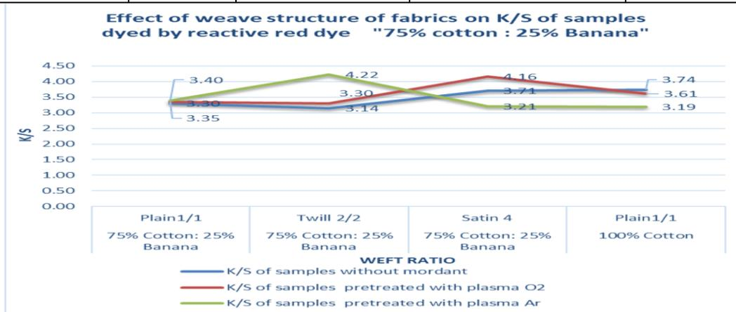
Fig. (16): Effect of weave structure of fabrics on K/S of dyed samples with Reactive red in presence and absence of plasma treatment.
