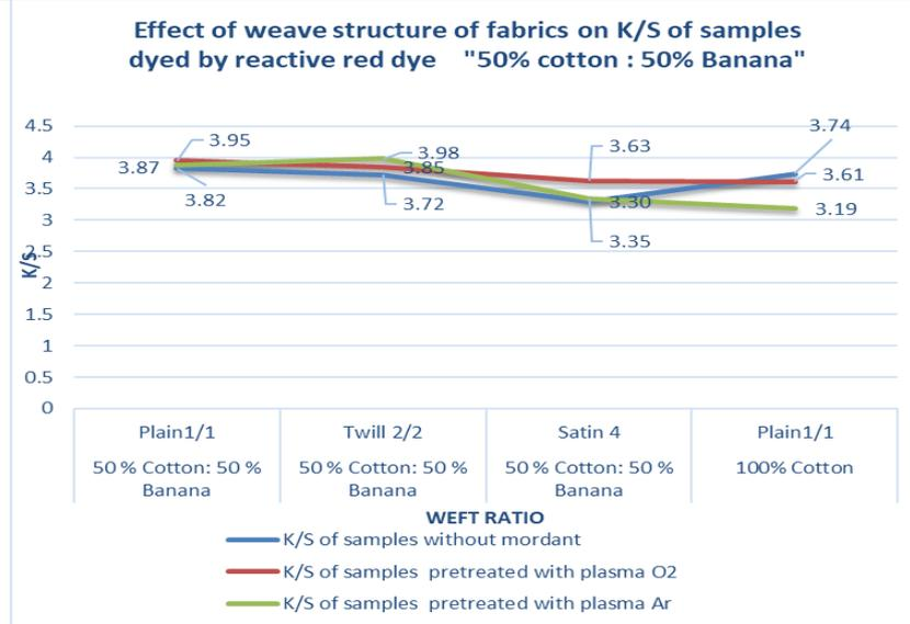
Fig. (18): Effect of weave structure of fabrics on K/S of dyed samples with Reactive red in presence and absence of plasma treatment.
