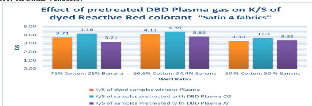
Fig. (15): Effect of using Pre-treatment plasma on dyeing Satin 4 fabrics with reactive Red dye in presence of different gases.
