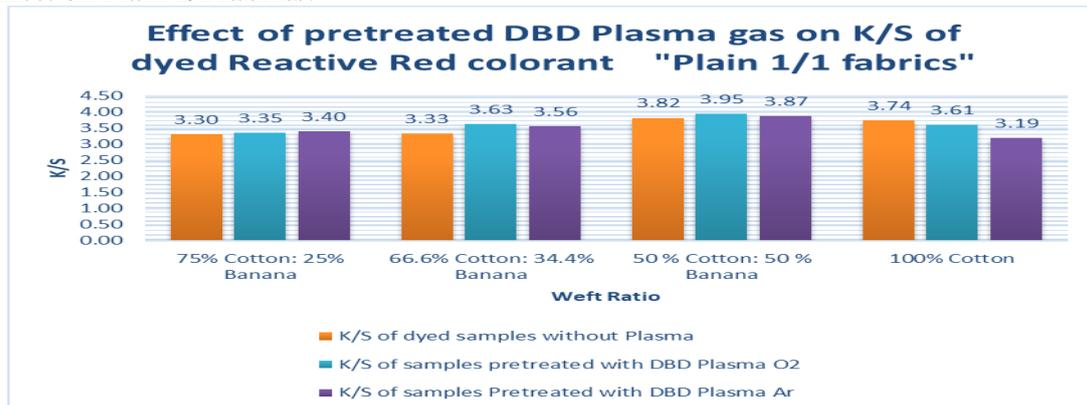
Fig. (13): Effect of using Pre-treatment plasma on dyeing plain fabrics with reactive Red dye in presence of different gases.
