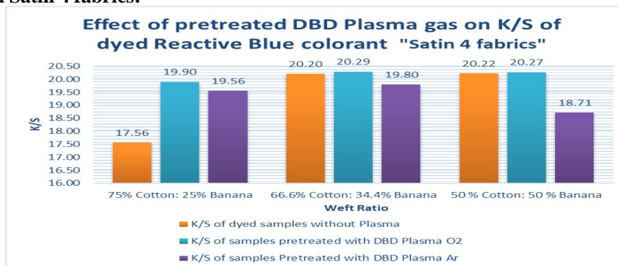
Fig. (9): Effect of using Pre-treatment plasma on dyeing Satin 4 fabrics with reactive blue dye in presence of different gases.
